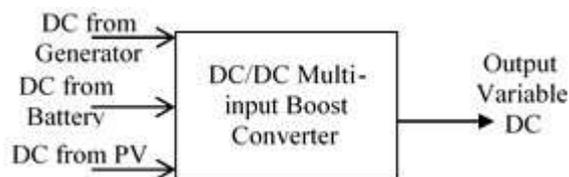
Fig. 2: Multi-input single output boost converter
