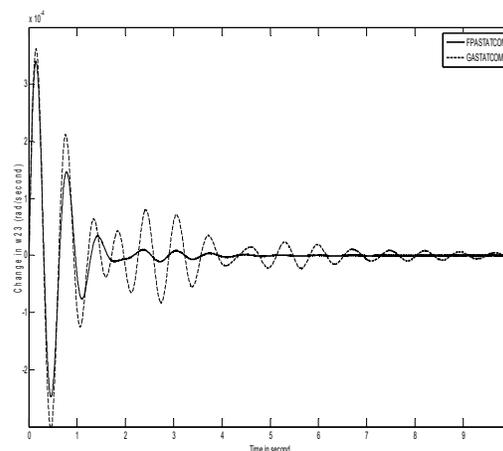
Fig. 10: Change of  $\Delta\omega_{23}$  under heavy condition.
