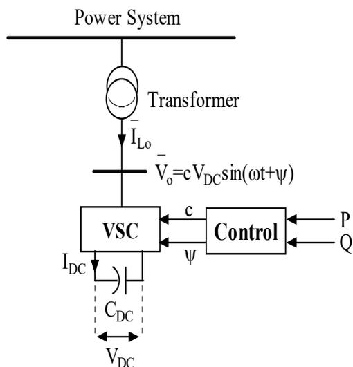
Fig. 1: Active and reactive power control of STATCOM.
