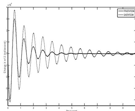
Fig. 9: Change of  $\Delta\omega_{12}$  under heavy condition.
