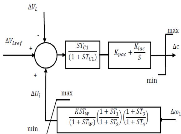
Fig. 3: Block diagram of AC voltage regulator with supplementary signal.
