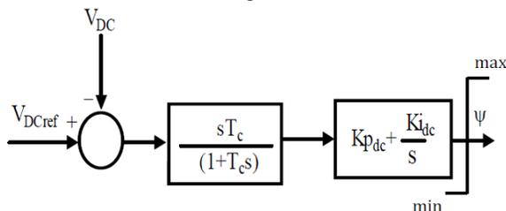
Fig. 2: Dynamic model of DC voltage regulator.
