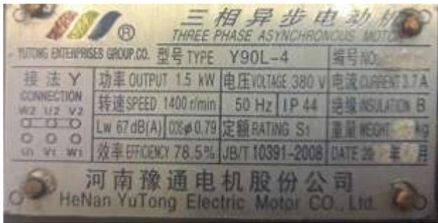
Fig. 1: Three phase Induction Motor name plate
