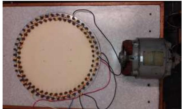
Fig. 2: Stator connection layout
