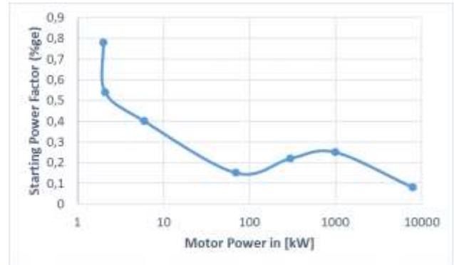
Fig. 9: Power factor start for different motors.
