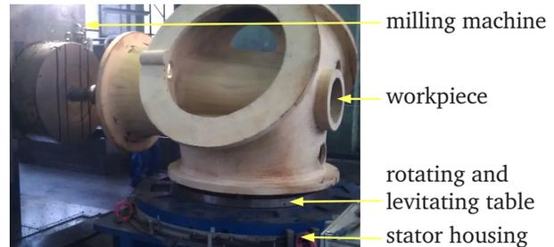
Figure 13: Workpiece milling on rotary table prototype 2 (RTP2) ( $m_w \approx 1900 kg$ )
