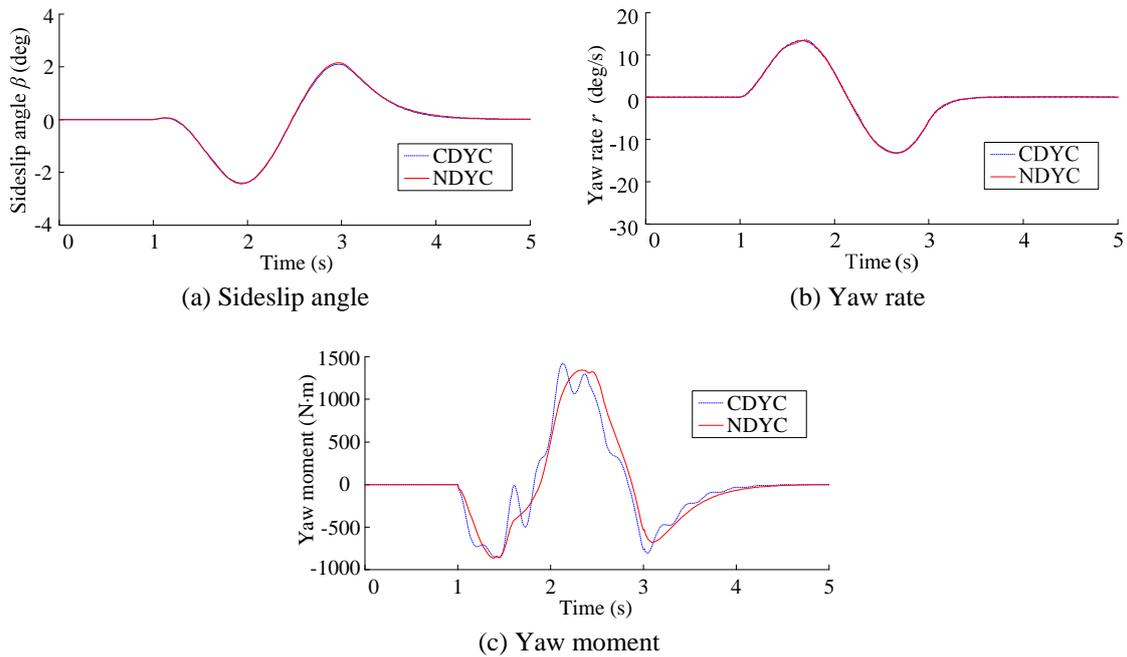
Fig.7: Comparison of vehicle responses with different control systems at pure time delay  $\eta = 0.01s$ .
