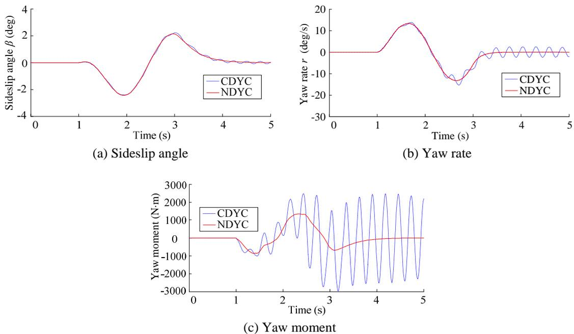
Fig.8: Comparison of vehicle responses with different control systems at pure time delay  $\eta = 0.02s$ .
