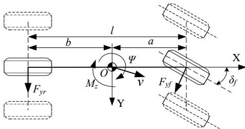
Fig. 2: 2DOF vehicle model
