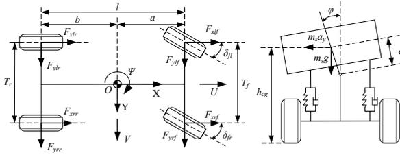
Fig. 1: SAE 8DOF Vehicle model
