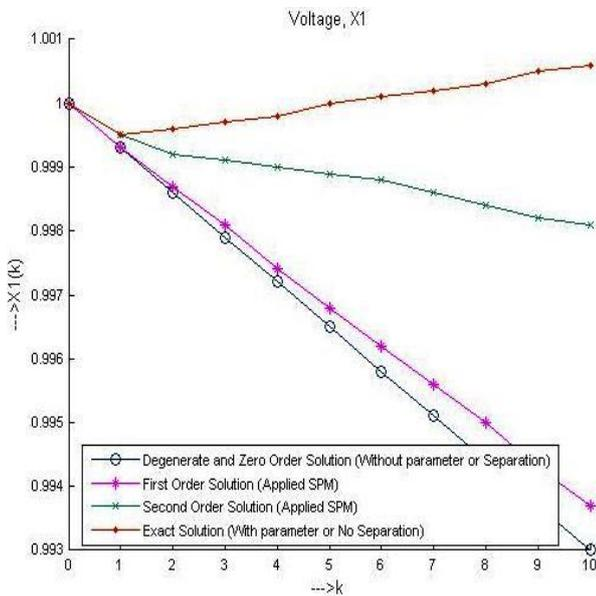
Graph .1: Comparison of various series solutions with the exact solution for voltage ( $X_1$  or  $x_0$ ) for IVP
