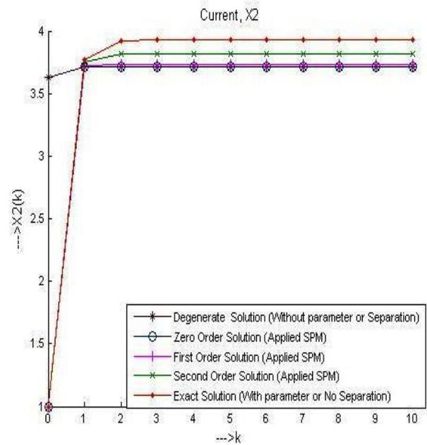
Graph .2: Comparison of various series solutions with the exact solution for current ( $X_2$  or  $x_1$ ) for IVP
