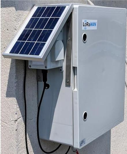
Fig. 5. A commercial AQI monitoring station of the “Paisii Hilendarski” University of Plovdiv, utilized by EMULSION (<https://smartcity.shieldo.space/>).
