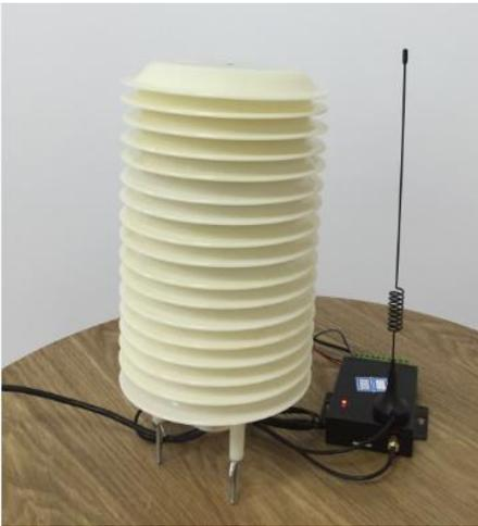
Fig. 6. A sample self-elaborated AQI monitoring station, utilized by EMULSION.
