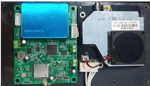
Fig. 7. A sample hardware of a self-elaborated AQI monitoring station, utilized by EMULSION.
