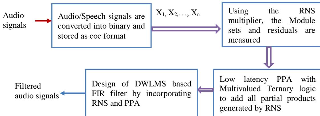
Fig. 4: Overall block diagram of FIR filter using Residual Number System filter with Parallel Prefix Adder for ECG signal applications
