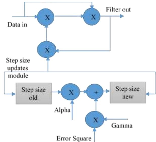
Fig. 1: Architectural diagram of 1-tap Coefficients used in FIR filter
