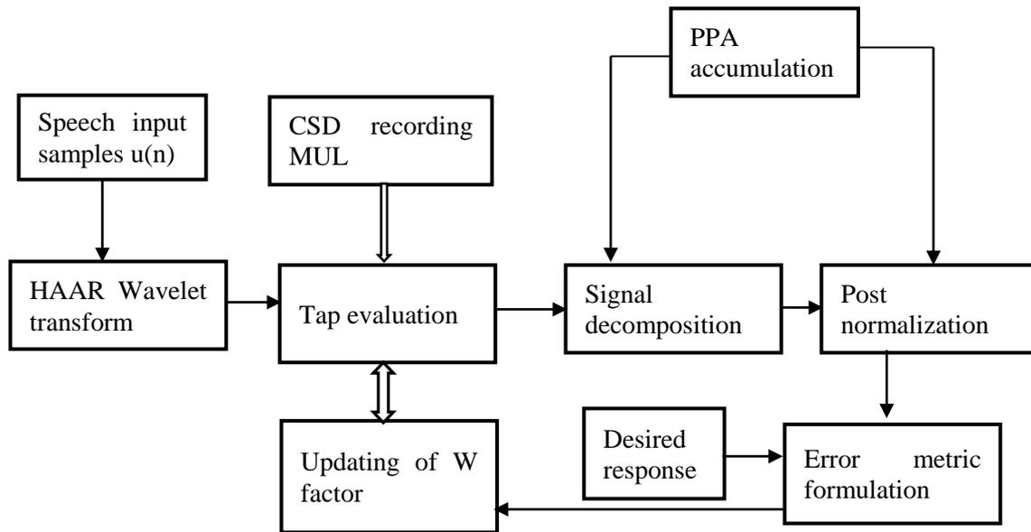
Fig. 2: Proposed wavelet transform domain used in NLMS architecture
