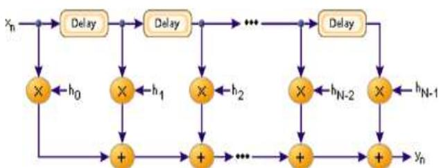
Fig. 3: A Finite Impulse Response filter's major infrastructure
