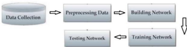
Fig. 1: Flowchart of building a Neural Network
