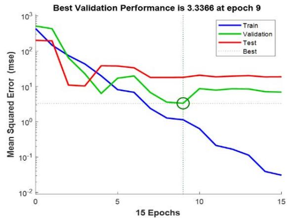
Fig. 9: Best validation performance of the SCG network for 150 neurons
