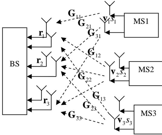
Fig.2 MIMO CR uplink base-band system
