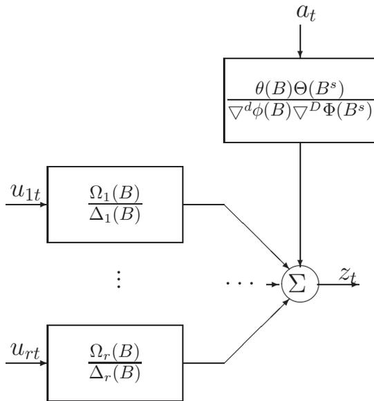
Fig. 2: Transfer function (*TF*) model
