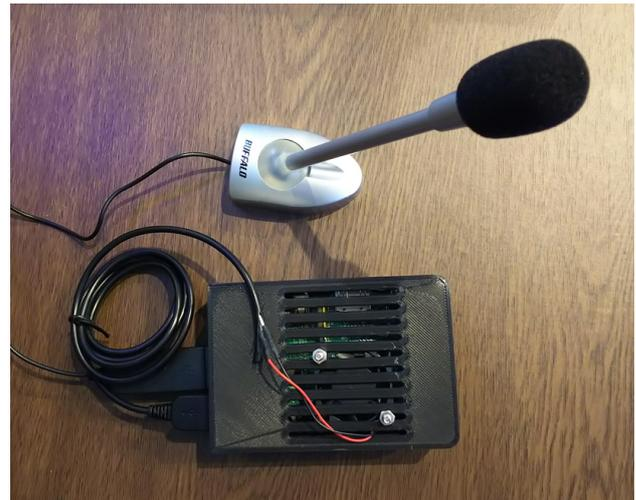
**Figure 5:** The developed prototype. The system is based on a Raspberry Pi running Ubuntu Server with an external USB microphone connected.
