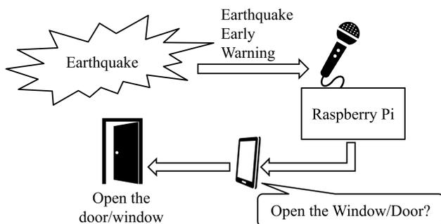
**Figure 4:** Overview of the proposed system. When an earthquake occurs and the reception of an Earthquake Early Warning is detected, a confirmation message is sent to the resident's smartphone, prompting whether to open windows or doors. The system will then execute the opening process based on the resident's input.
