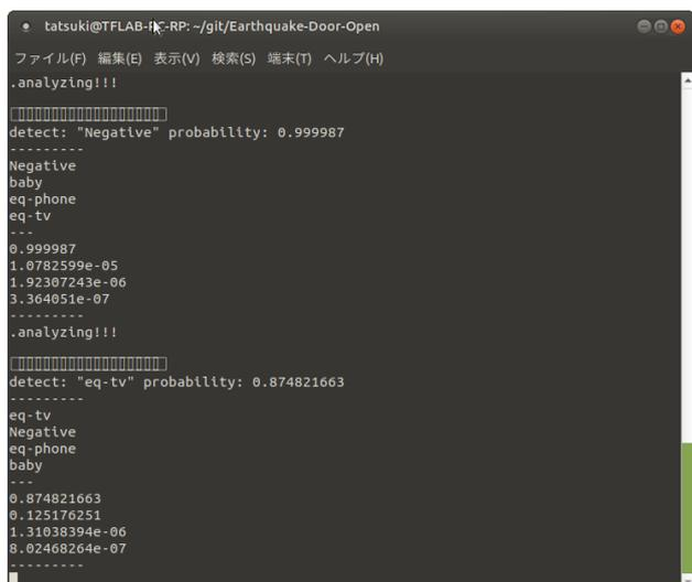
**Figure 6:** Screenshot of the program in operation. The audio input from the microphone is classified into four categories: Earthquake Early Warning from smartphone (eq-phone), Earthquake Early Warning from television (eq-tv), baby crying (baby), and other sounds (Negative).
