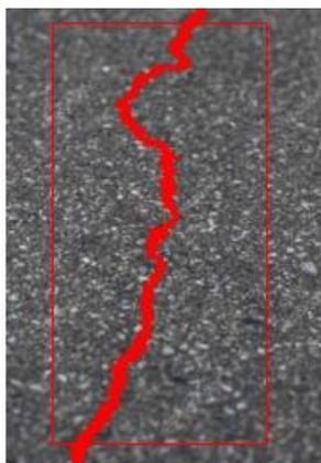
Fig. 5: Results of crack detection
