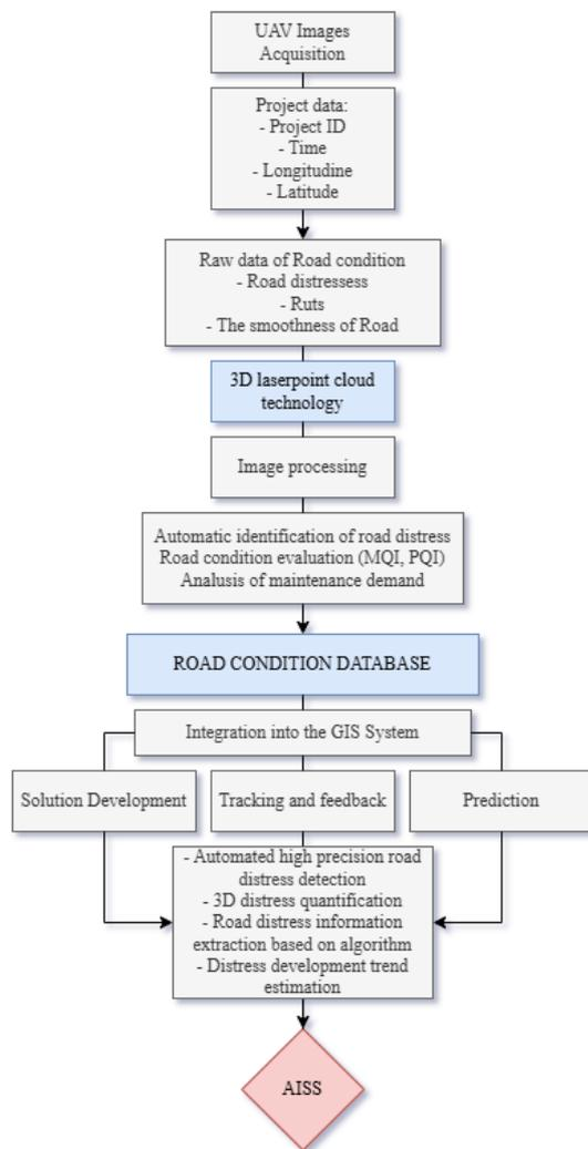
Fig. 1: Methodology of the experimental proposed system for road monitoring
