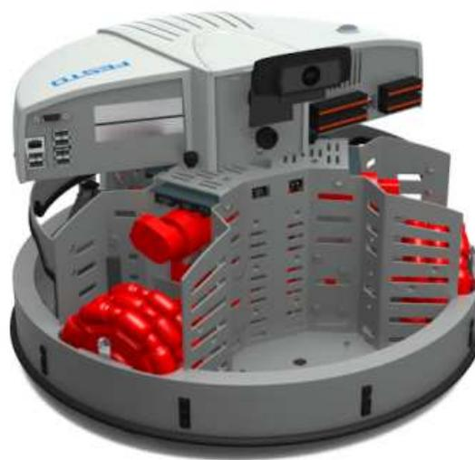
Fig. 1. Festo Robotino Mobile Robotic Development Platform
