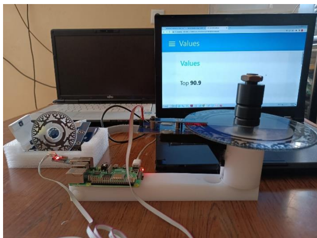
Fig.12 Disk of Gray code attached to raspberry computer and wireless connection with laptop.
