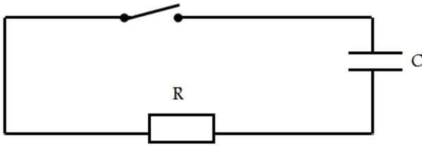
Fig. 5: Diagram of RC circuit in the absence of a voltage source.
