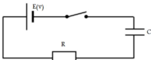
Fig. 4: Diagram of RC circuit in the presence of a voltage source.
