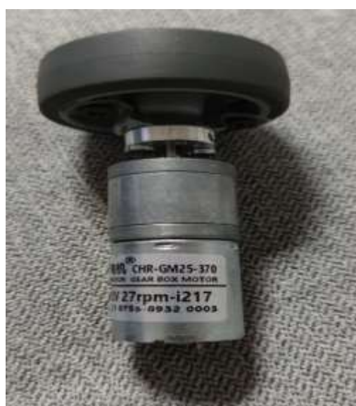
Fig. 4: The gear motor, DC, CHR-GM25-370-12V 27 RPM
