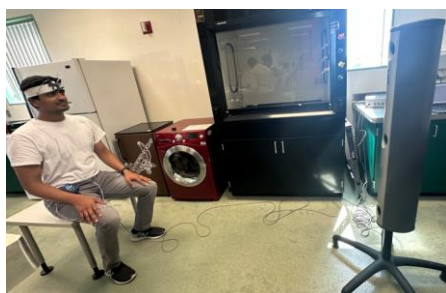
The device setup including the OC3D tower, OC3D reflective markers on the forehead, and the IMU at the back of the head.
