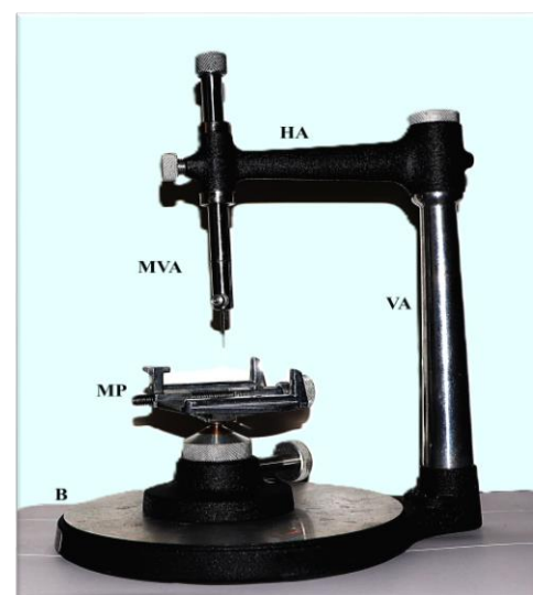
Fig. 3: The classical surveyor main components VSA; vertical axis, HA; horizontal axis, MVA; movable vertical axis, MP; movable plate, B; base of surveyor
