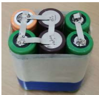
Fig. 7. The battery pack has a capacity of 12V dc
