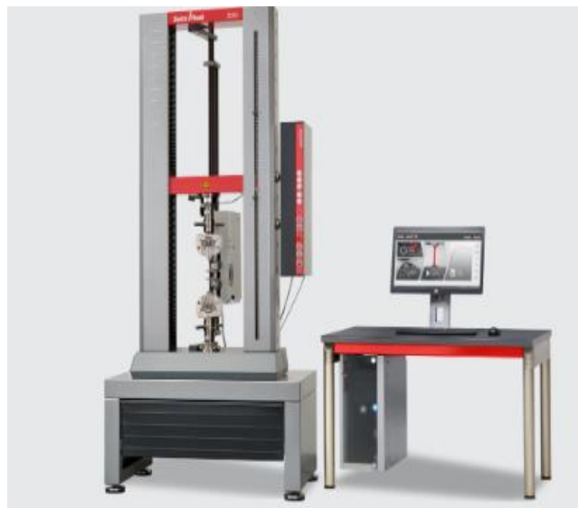
Figure 1. Zwick Roell Z100 universal mechanical testing machine.
