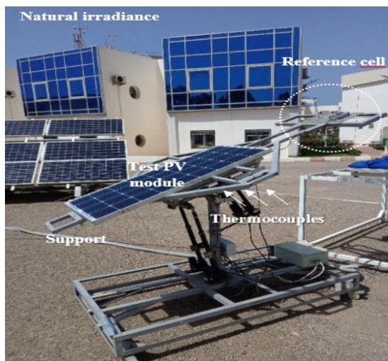
Fig. 2 Sun-tracking structure for the tested PV module
