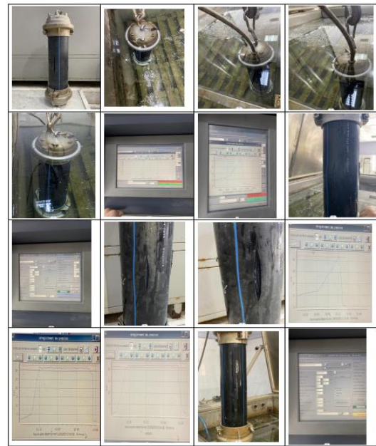
Fig. 3: Illustrates burst tests performed on the TUBEX test bench Source: Created by the authors
