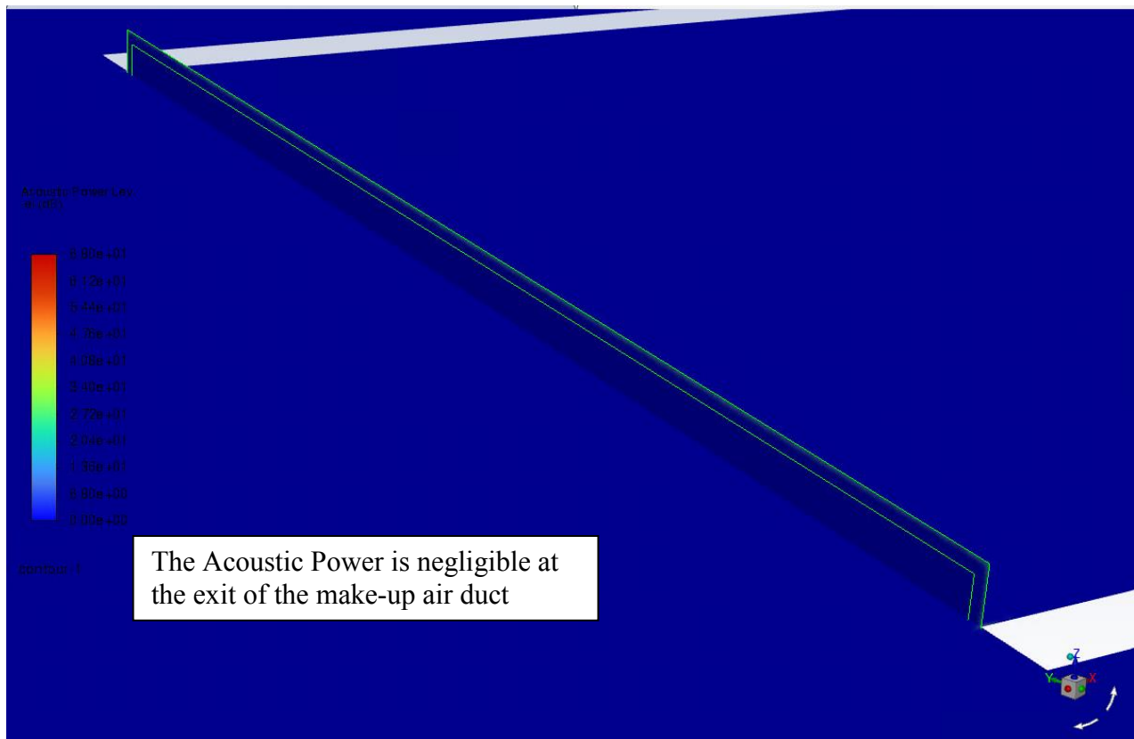
Fig. 11: Acoustic Power Level (dB) at the Exit of the Make-up Air Duct, Motorised Damper is Fully Open, Exhaust fans are operated, and ALL doors and Windows are closed Source: developed by the author
